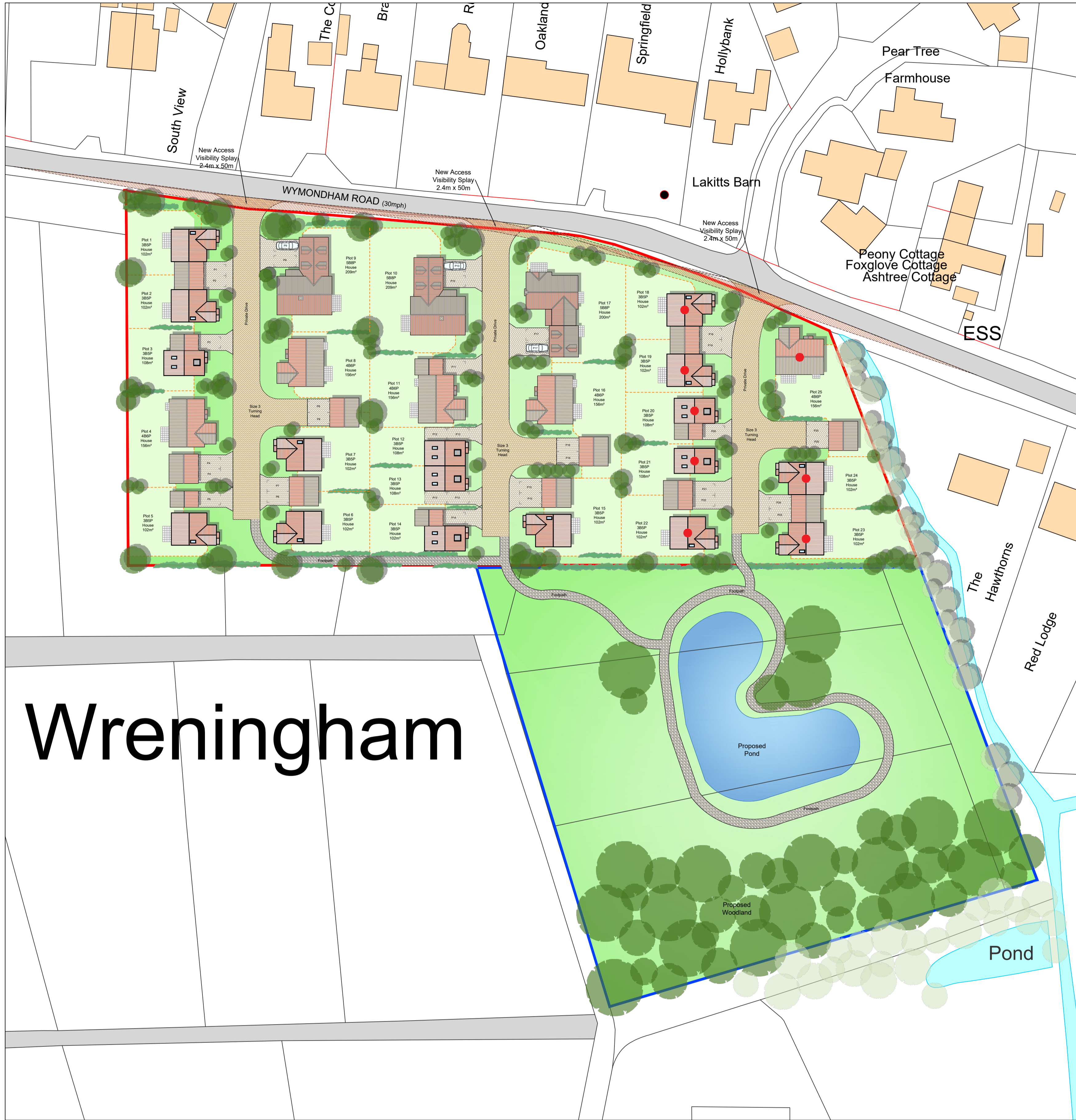
Proposed Site Layout Plan 1:500 0m 10m 20m 30m 40m 50m
