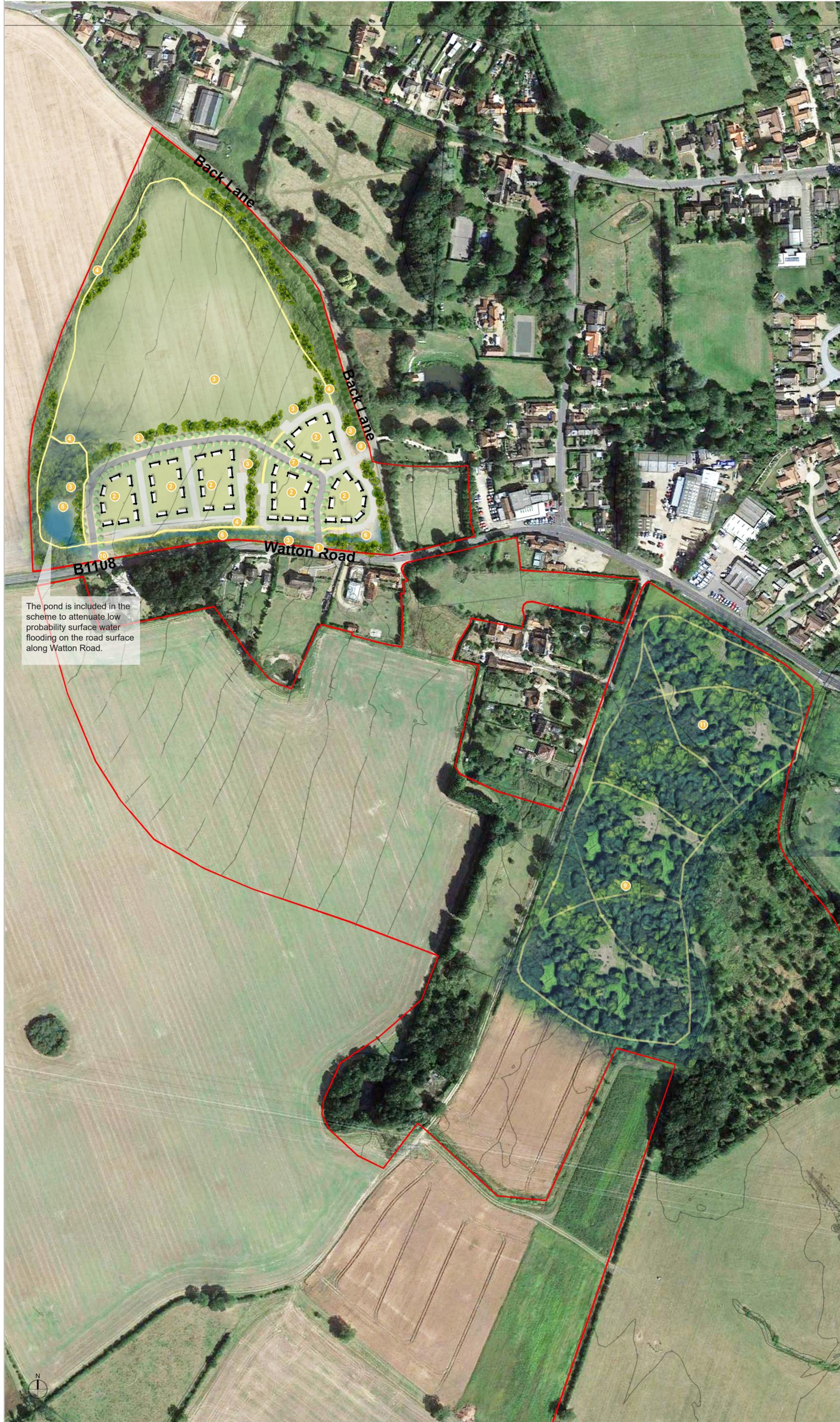
The pond is included in the scheme to attenuate low probability surface water flooding on the road surface along Watton Road.
