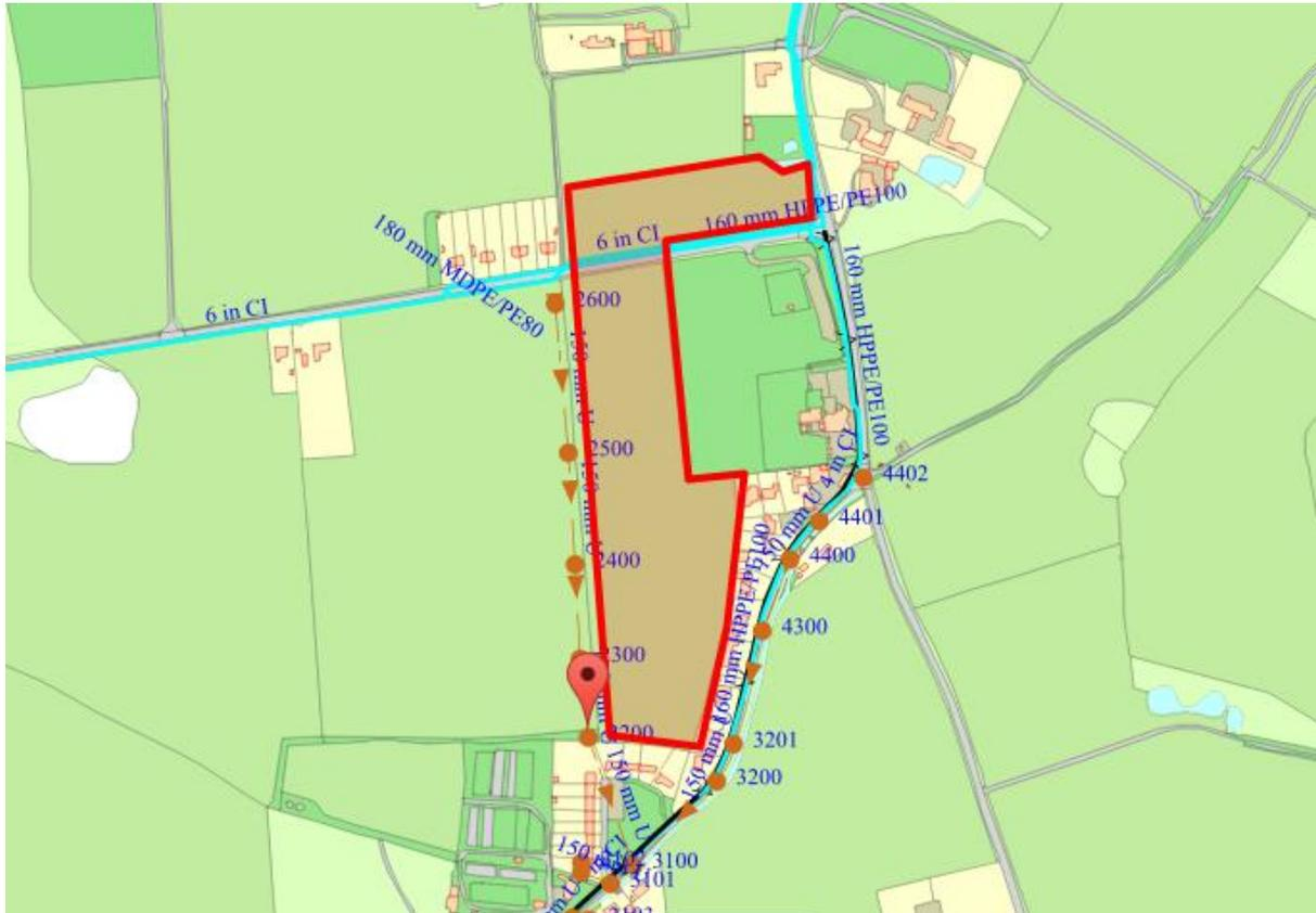
Figure 1: Your used water point of connection at manhole 2200
